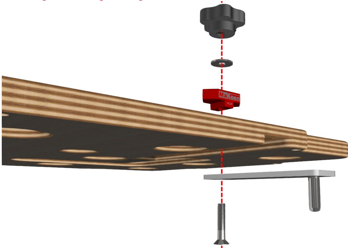
Figure1 - Insertion sequence of the sliding carriage in the MFT template
