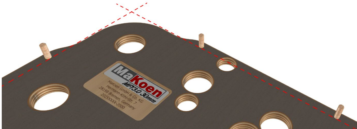
Figure 11 : Stop edge formed by pins
