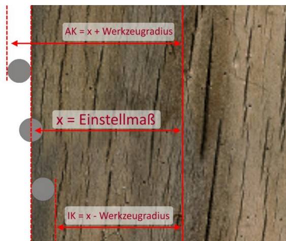
Figure 4- Illustration of outer contour to inner contour
